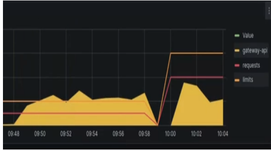
Fig. 9. Graphical representation of network policy adaptation showing CPU usage in cores for the Gateway API pod (yellow line), requested CPU (red line), and CPU limits (orange line) over time. The graph illustrates a restart period with no CPU usage, followed by increased resource utilization after the application of a new policy that allowed more CPU resources.
