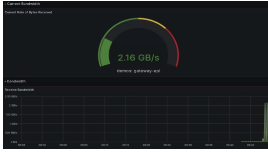
Fig. 8. The bandwidth of the Gateway API pod after the applied policy. The capacity of bandwidth is increased to support the increased demand where the received bandwidth goes from 30MB/s to 2GB/s.
